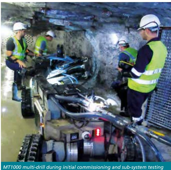
MT1000 multi-drill during initial commissioning and sub-system testing
