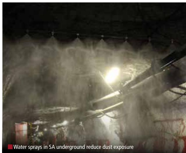
Water sprays in SA underground reduce dust exposure
